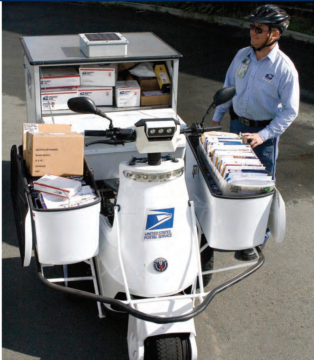
The T3 electric delivery vehicle and cart can carry up to 450 pounds of mail and costs 2 cents a mile to operate.
